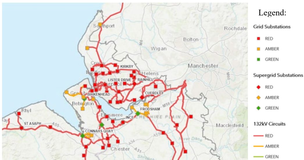
Figure 5.2: SPM's HV distribution network capacity for connecting generation (source: SPEN's heat map).
