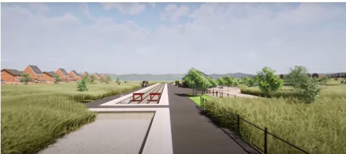
Figure 10.4: At-grade step-free crossing
